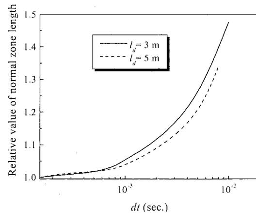
Fig. 3 Relative values of maximum pressure, normal zone length versus time step. The values calculated by  $\Delta t = 0.1$  ms and  $\Delta x = 3.5$  mm is employed as the reference values.
