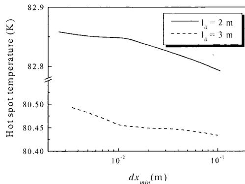
Fig. 2 Hot-spot temperature profiles versus space interval, we assume the time stepsize to be kept constant  $\Delta t = 0.1$  ms.
