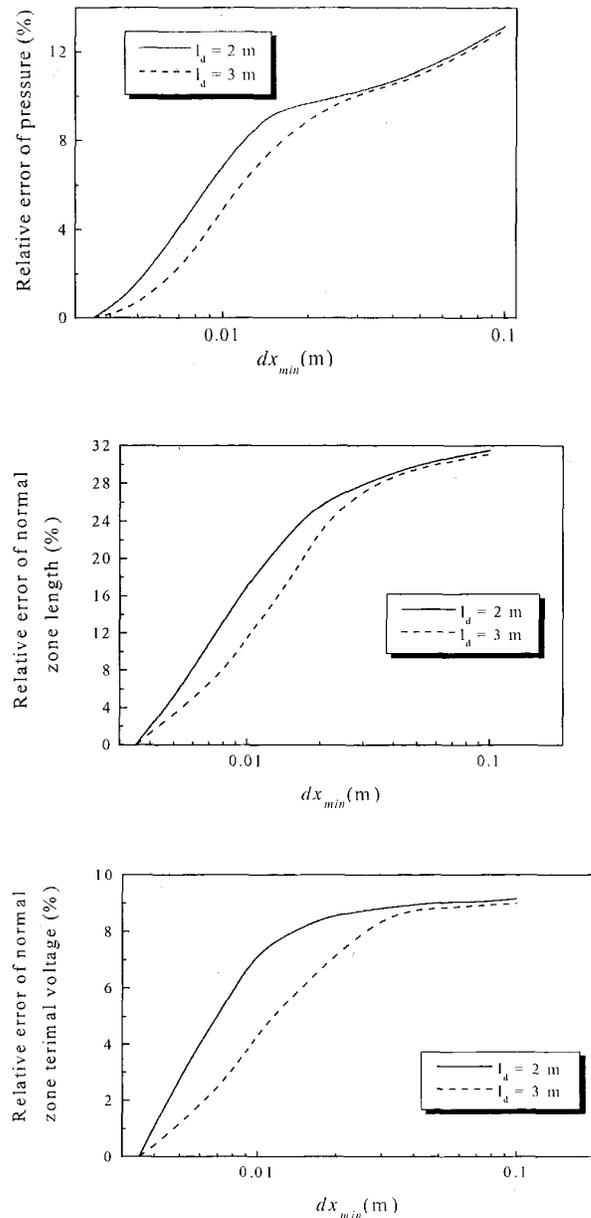
Fig. 1 Relative error profiles of maximum pressure, normal zone length and voltage of normal zone terminate versus space step. The values calculated by  $\Delta t = 0.1$  ms and  $dx_{min} = 3.5$  mm are used as the reference values.
