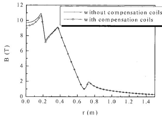
Fig. 3 Magnetic field distribution of SSTF background magnet system along the R-direction for  $z = 0.38$  m, with and without compensation coils.
