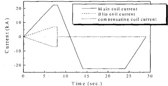
Fig. 5 Operating current versus time in SSTF system.
