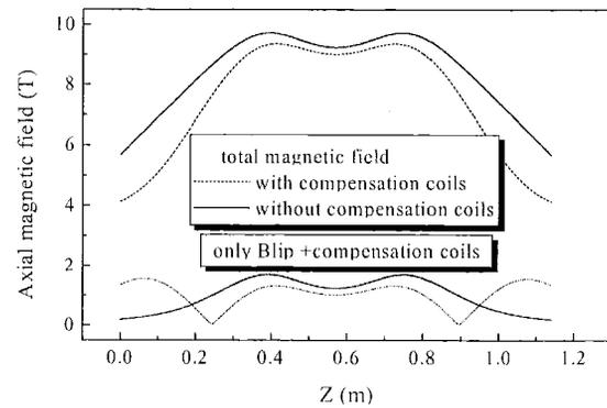
Fig. 2 Magnetic field distribution with compensation coils and without compensation coils in the axis of SSTF.
