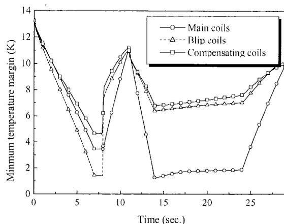
Fig. 8 Temperature margin in SSTF for operating condition for the system as Fig.7.
