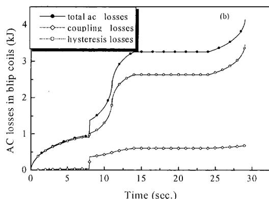
Fig. 6 AC losses in SSTF of the operating current shown in Fig.5.
