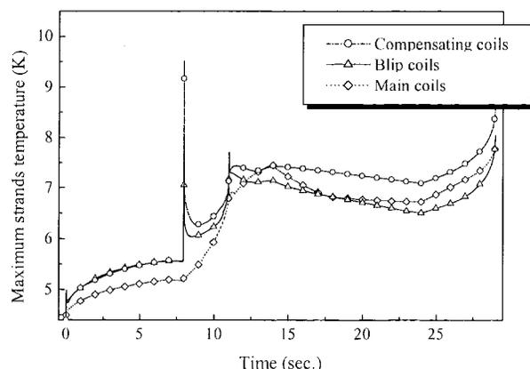
Fig. 7 Temperature rise in SSTF for inlet and outlet pressures of 0.6 and 0.3 MPa and inlet temperature of 4.5 K for main coils and 4.4 K for the blip and compensating coils.
