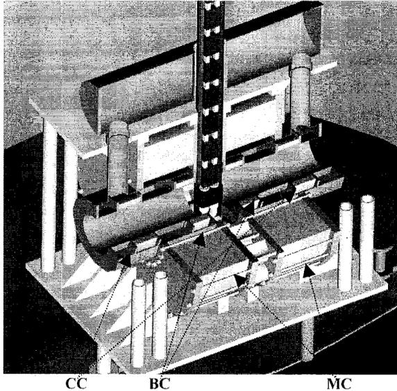
Fig. 1 Configuration of Samsung Superconducting Test Facility (1, 2-Main coils-MC, 5,6 -compensating coils-CC,3,4-blip coils-BC).
