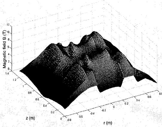
Fig. 4 Overall magnetic field ( $B$ ) distribution for SSTF with operating current 22.38 kA in the background magnets.
