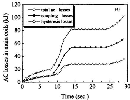
Fig. 3. Coupling, hysteresis and total losses in main coils with respect to time.
