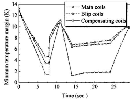
Fig. 4. Temperature margin in SSTF for given operating condition.
