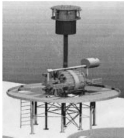
Fig. 1. Configuration of SSTF, which includes transformer, supporting structure, main, blip and compensating coils.
