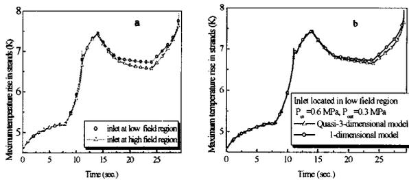
Fig. 9. Maximum peak temperature of main coils versus time for inlet pressure of 0.6 MPa and outlet pressure of 0.3 MPa, and helium inlet located in the low field region and the high field region (a) for various heat transfer models such as 3-d and 1-d (b).
