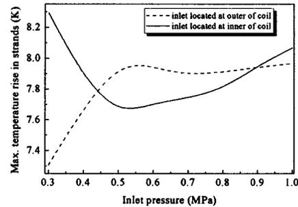
Fig. 8. Variation of the maximum peak temperature rise in superconducting strands with inlet pressure and positions for the outlet pressure kept in constant of 0.3 MPa.
