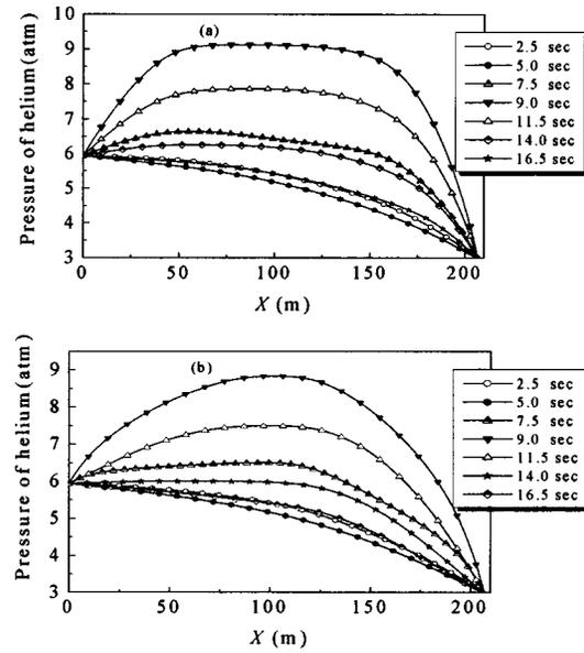
Fig. 7. Profiles of pressure of helium with respect to space coordinate for inlet pressure of 0.6 MPa and outlet pressure of 0.3 MPa, (a) helium inlet located at the low field region and (b) helium inlet located at the high field region.
