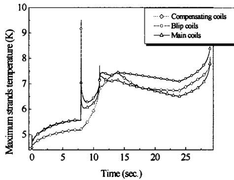
Fig. 2. Profiles of maximum peak temperature of superconducting strands versus time for the main, blip and compensating coils.
