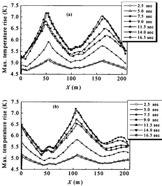
Fig. 6. Profiles of superconducting strands temperature versus space coordinate for inlet pressure of 0.6 MPa and outlet pressure of 0.3 MPa. (a) helium inlet located at the low field region and (b) helium inlet located at the high field region.
