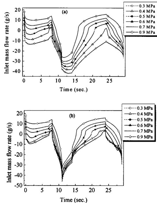
Fig. 5. Inlet mass flow for various inlet pressures and inlet positions in the main coils, the outlet pressure of 0.3 MPa, (a) helium inlet located at the low field region and (b) helium inlet located at the high field region.
