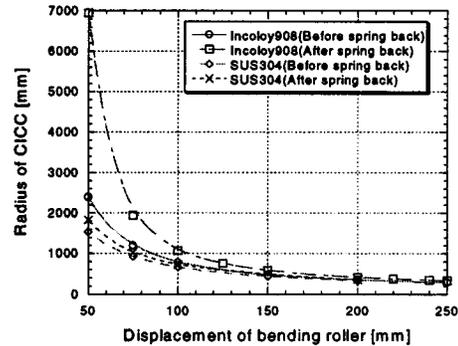
Fig. 5. Predicted radius of formed CICC after spring back versus displacement of the bending roller for both Incoloy 908 and SUS304. Monitoring points were taken near the master rollers.
