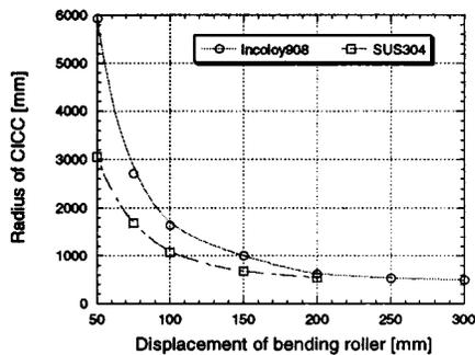
Fig. 6. Predicted radius of formed CICC after spring back versus distance of the bending roller for both Incoloy 908 and SUS304. Monitoring points were taken near the bending rollers.
