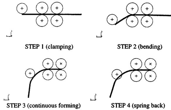
Fig. 4. Stepwise-deformed shape of CICC with downward bending roller travel of 200 mm (Material: Incoloy 908).
