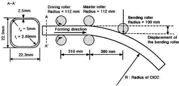
Fig. 3. Schematics of 3-roll bending process to form CICC.
