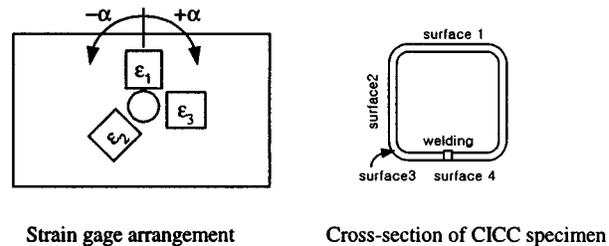
Fig. 8. Schematic of strain gage arrangements and locations.
