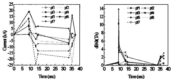
Fig. 3. Operating current and  $dB/dt$  in PF coils.
