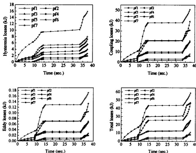
Fig. 5. Hysteresis, coupling, eddy currents and total AC losses in PF coils.
