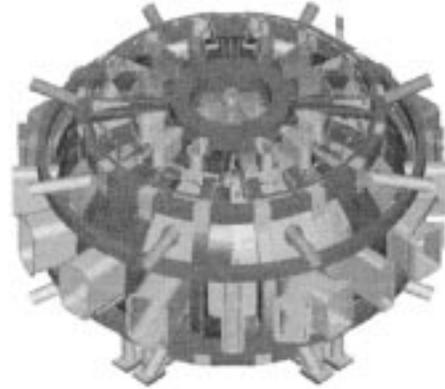
Fig. 1. PF, TF coils, support structures, and vacuum system of KSTAR.
