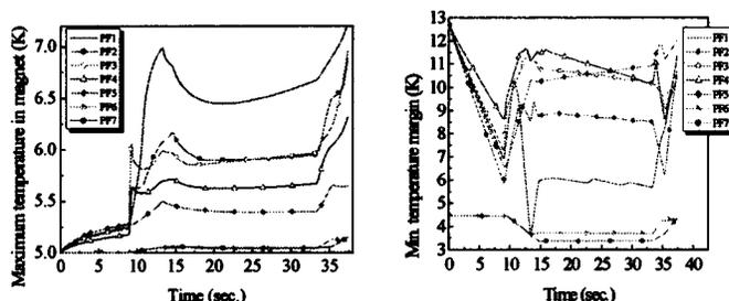
Fig. 6. Maximum temperature rise and temperature margin for PF coils during normal operating scenarios.
