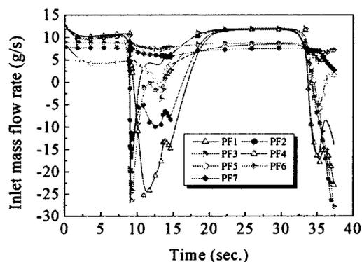
Fig. 7. Inlet mass flow rate with respect to time, during the plasma discharging interval of the KSTAR operating scenario.
