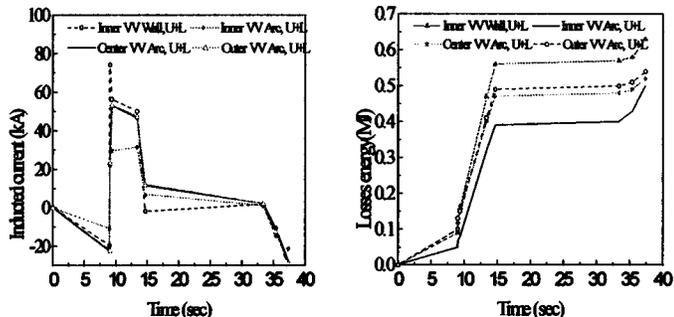
Fig. 4. Induced current and losses energy in the passive structure (VV: vacuum vessel, U: upper, L: lower).
