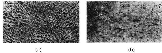
Fig. 3. The microstructure of Incoloy 908 weld (Weldment) (a) and heat affected zone (HAZ) (b).
