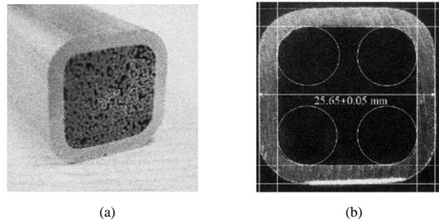
Fig. 2. TF 01 CICC (a) and the cross section appearance (b).
