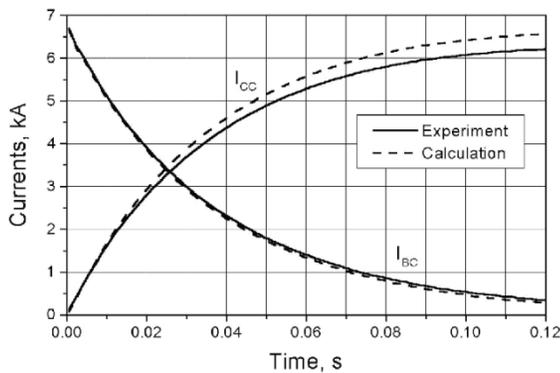
Fig. 6. BC self-field test: fast discharge and PCC charging.
