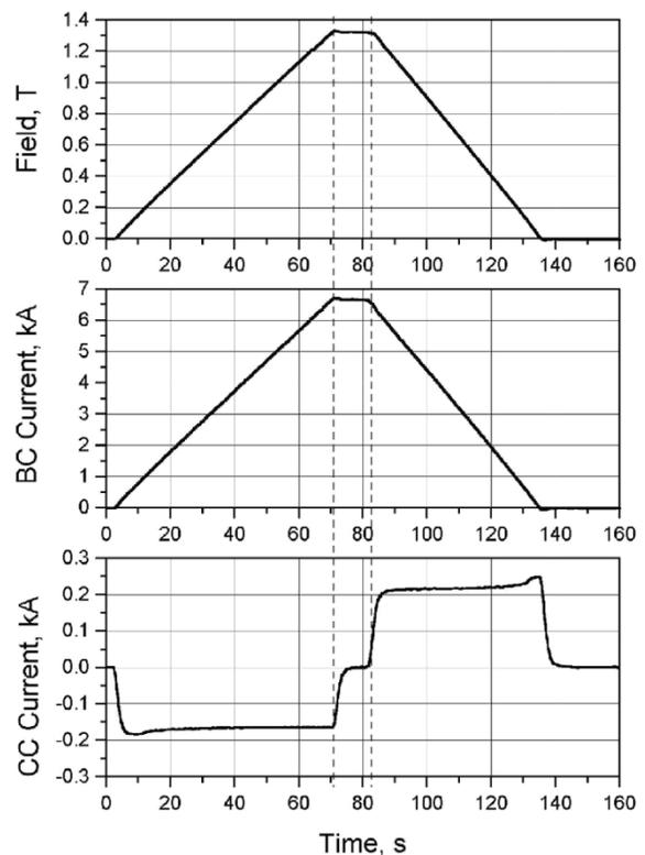
Fig. 5. BC self-field test: slow charging with PCC short circuited.
