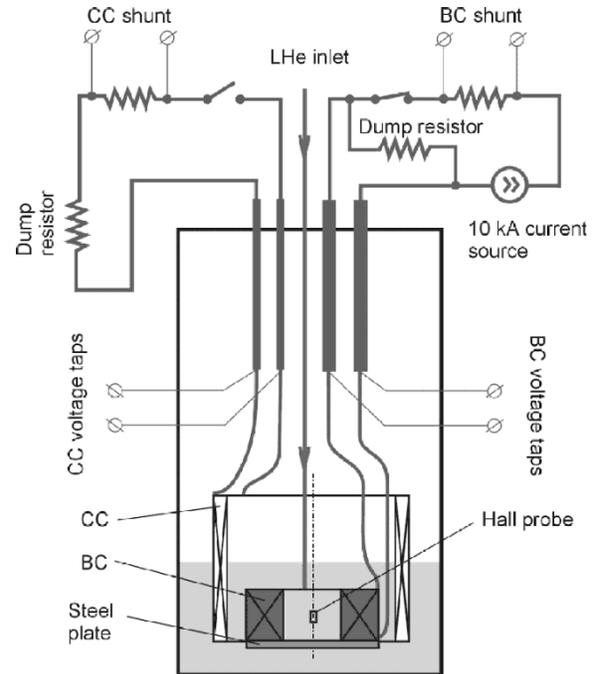
Fig. 4. Schematic diagram for the test of BC and PCC.
