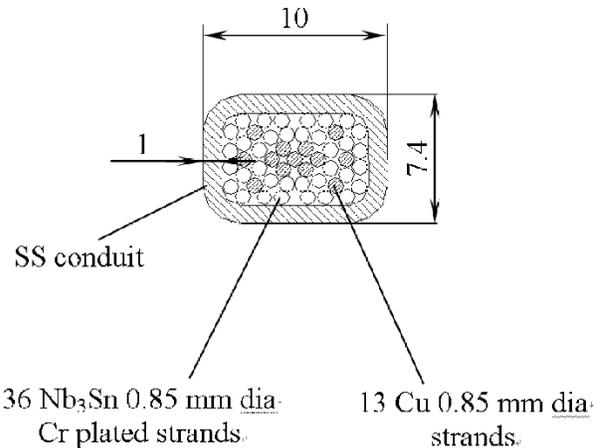
Fig. 1. BC conductor cross-section (unit: mm).
