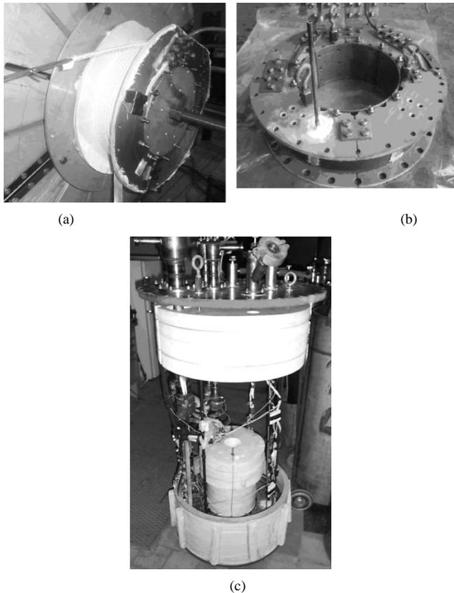
Fig. 3. BC coil fabrication: (a) winding with insulated CICC, (b) installation of fiber glass flanges after the reaction, and (c) test preparation of BC and PCC after the impregnation.
