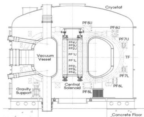
**Fig.2** KSTAR superconducting magnet system configuration
