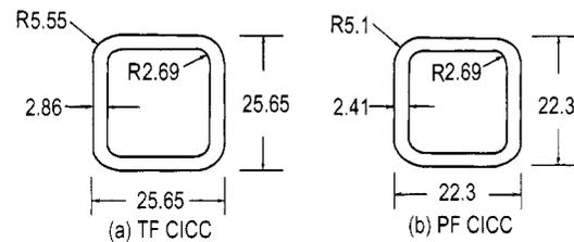
**Fig.3** Dimension of TF (a) and (b) CICC
