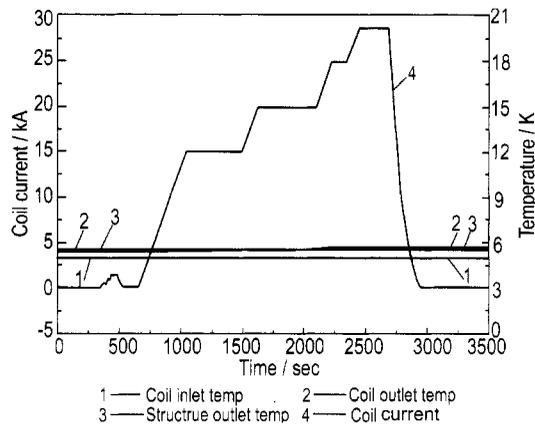
Fig.6 Current ramping and discharge of TF00
