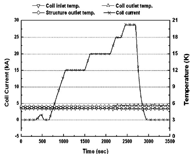
Fig. 4. Current ramp up to 29 kA and slow discharge.
