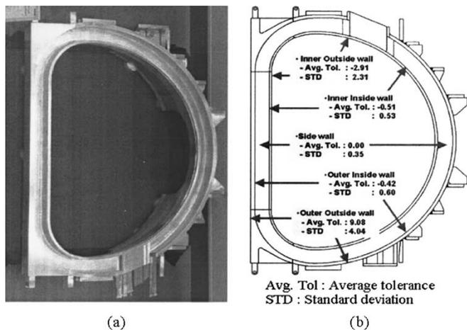
Fig. 3. Prototype TF structure. (a) Prototype TF structure case. (b) Dimensional measurement results of prototype TF structure case.
