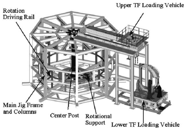
Fig. 6. Schematic 3-D view of main jig system for TF assembly.
