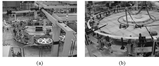
Fig. 2. Winding station for TF and PF coils. (a) TF winding. (b) PF7L winding.
