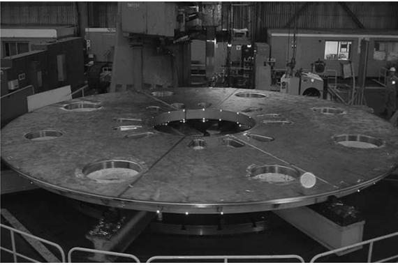
Fig. 5. Machining of cryostat base plate (May 12, 2003).
