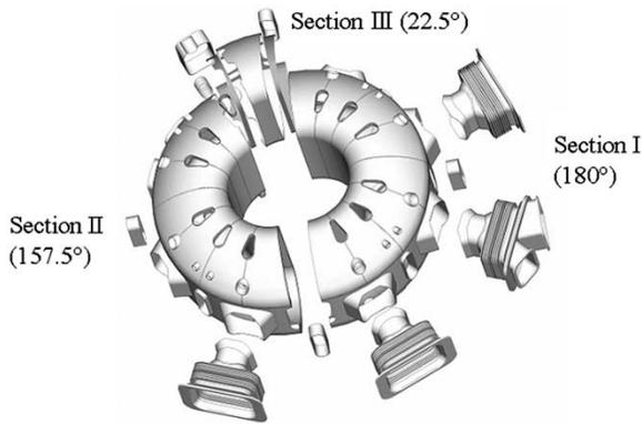
Fig. 1. Vacuum vessel segmentation.
