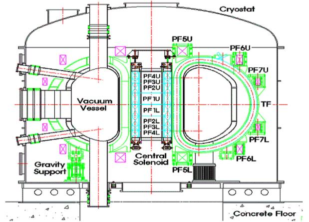
Fig. 2. KSTAR superconducting magnet system configuration.
