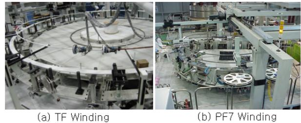
Fig. 4. Winding Station for TF and PF coils.
