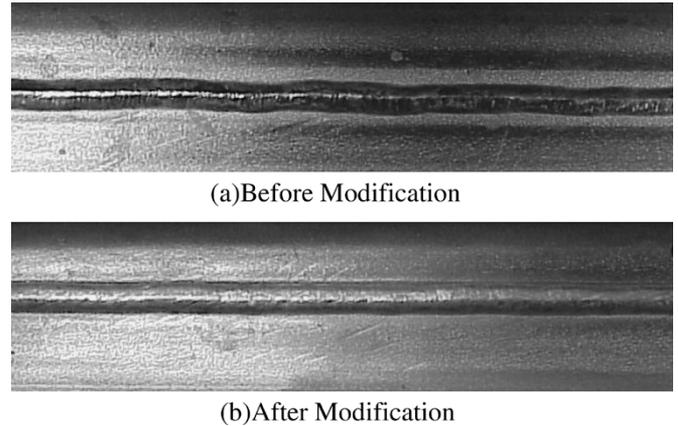
Fig. 5. Welding back bead (a) before modification, (b) after modification.
