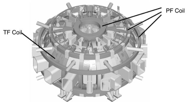
Fig. 1. Arrangement of the KSTAR magnet system.
