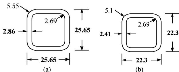
Fig. 2. Final dimension of conduits for TF and PF CICC (unit: mm). (a) TF CICC; (b) PF CICC.
