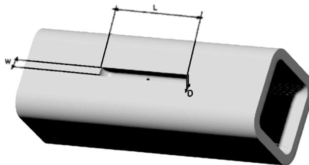
Fig. 3. CICC Sample for repair test (W: width, L: length, D: depth).
