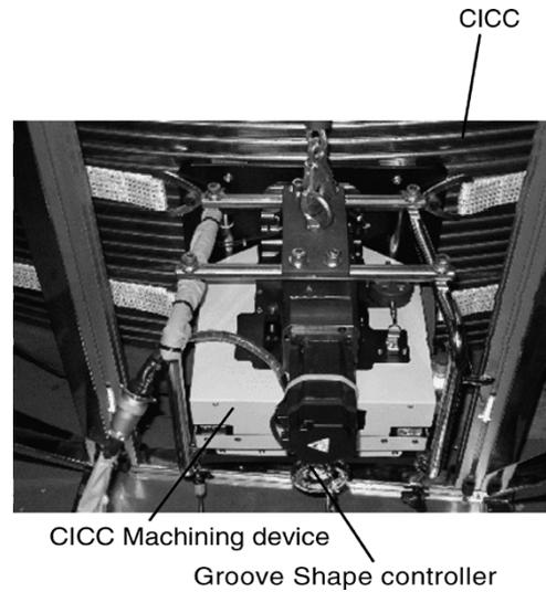
Fig. 4. CICC machining device for repair.
