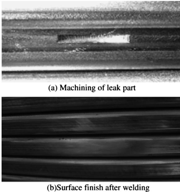
Fig. 6. Machining (a) and surface finishing part (b) of repair process.
