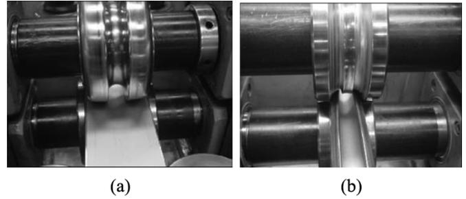
Fig. 1. The breaker pass and fin pass for tube forming. (a) Breaker pass; (b) fin pass.
