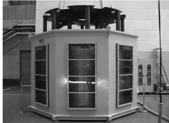
Fig. 4. Water chamber for the CICC leak check.
