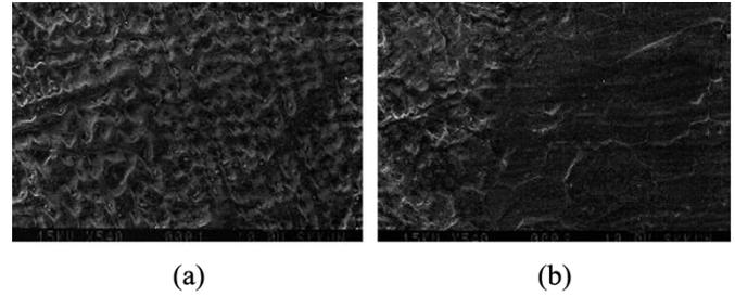
Fig. 3. The microstructure of Incoloy 908 weld (a) and heat affected zone (b).
