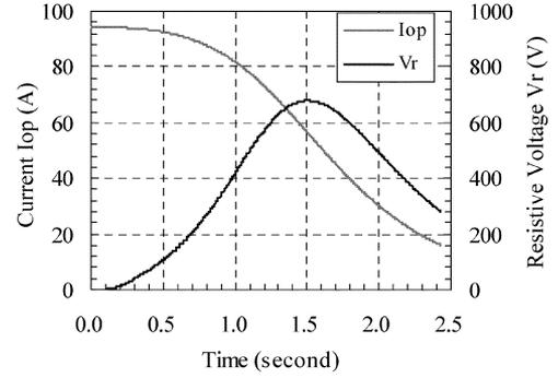
Fig. 8. Current and voltage versus time after quench.
