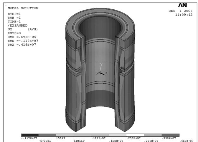
Fig. 5. Hoop stress distribution in superconducting magnet (Unit: Pa).
