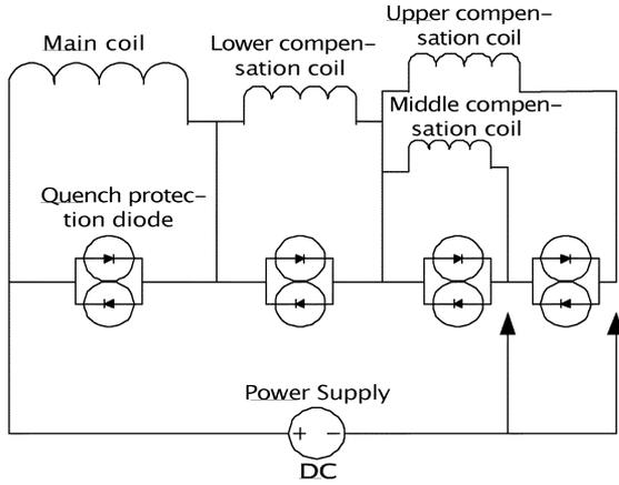
Fig. 6. Quench protection circuit of the superconducting magnet and current leads for two homogenous regions with length of 150 mm and 250 mm.
