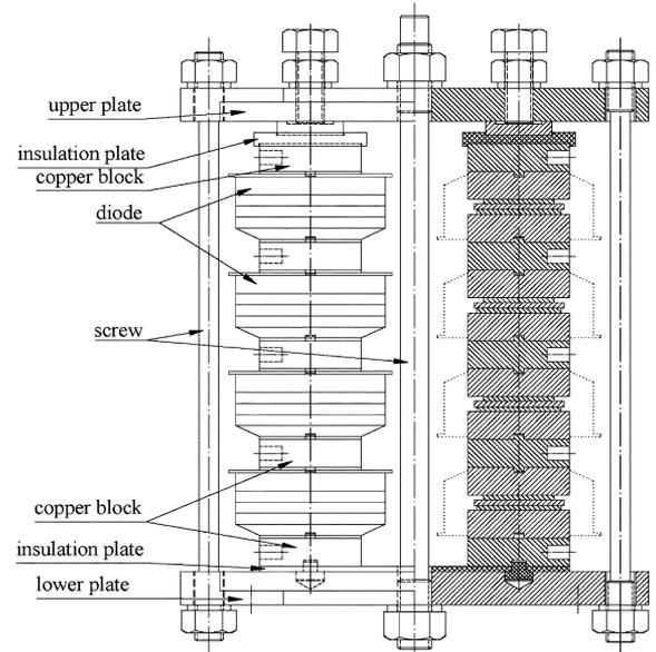
Fig. 9. Configuration of protection diodes and resistors in the magnet system.
