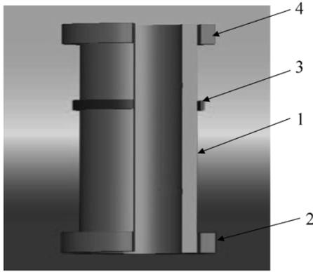
Fig. 2. Arrangement of coils for conduction-cooled magnet in gyrotron.
