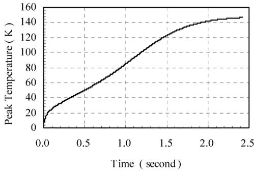
Fig. 7. Hot spot temperature rise in superconducting magnet.
