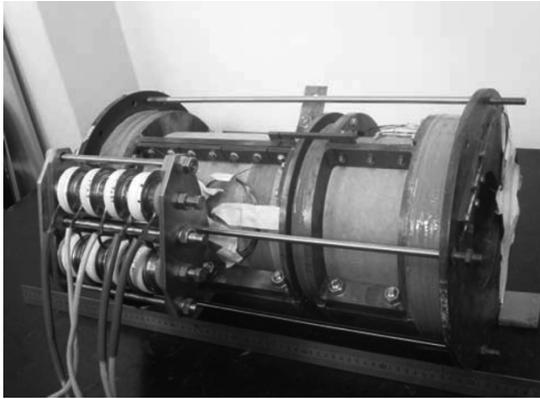
Fig. 10. Configuration of completed coil fabrication.
