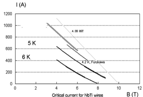
Fig. 1. Short sample characteristic for  $\varphi$  0.85 mm NbTi wire in various temperatures.
