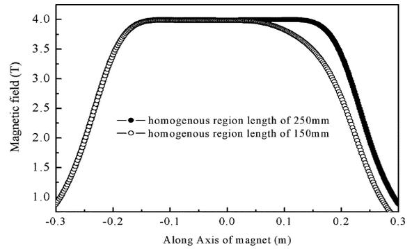
Fig. 3. Field distribution along the axis for two homogeneous regions.
