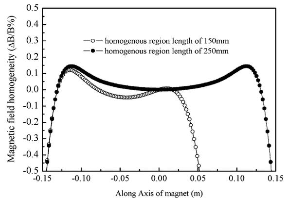
Fig. 4. Field homogeneity along the axis for two homogeneous regions.
