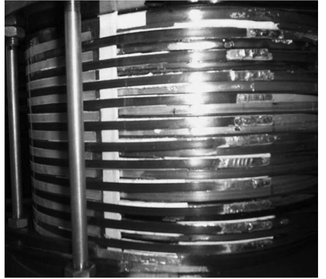
Fig. 3. Configuration of model high temperature coils.
