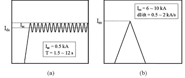
Fig. 3. Pulses for the AC loss analysis: Discrete values for  $T$  and  $dI/dt$  were used for the measurement. (a) DC-biased sine pulse; (b) singular triangular pulse.
