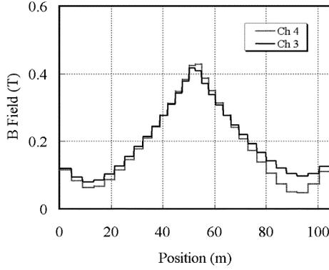
Fig. 4. Magnetic field profile along Ch3 and Ch4 of MC1 which was used for the AC characteristic analysis of the KSTAR CSMC:  $I_{op} = 1$  kA.
