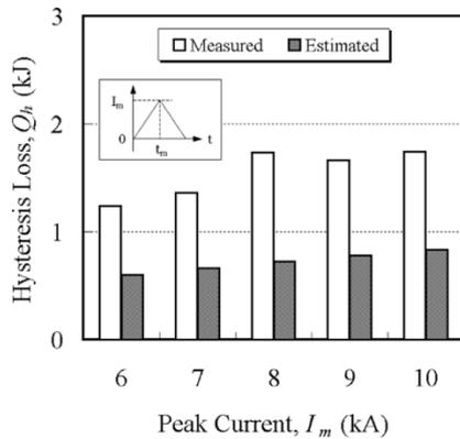
Fig. 7. Measured and estimated hysteresis loss in case of a single triangular pulse application.
