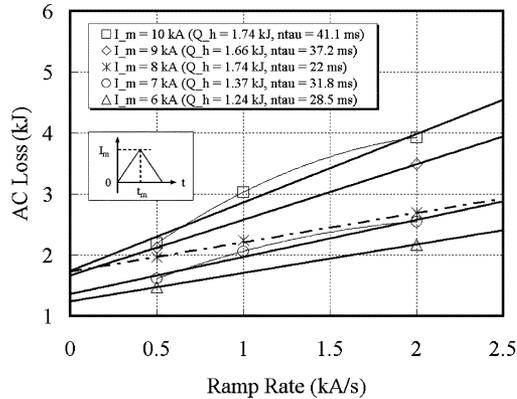
Fig. 6. Measured AC loss with the variation of the ramp rate of a single triangular pulse: Data was fit to straight lines to get the AC loss parameters and to curved lines to analyze the hysteresis loss in detail. In case of 8 kA, fit is expressed with a dotted line since it deviated from the normal trend.
