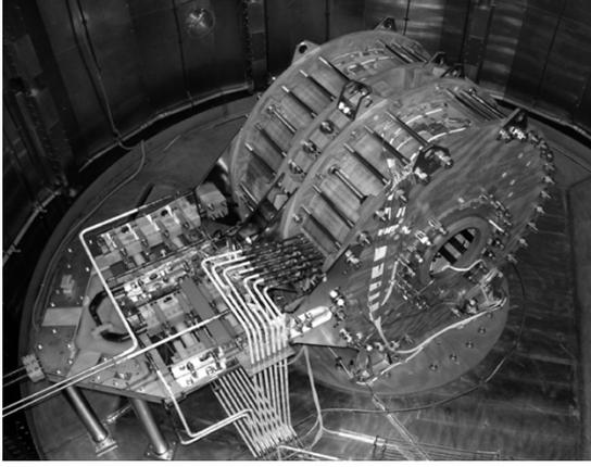
Fig. 1. KSTAR CSMC installed inside the large vacuum cryostat. The coil system consists of two split coils, MC1 (right side) and MC2 (left side).
