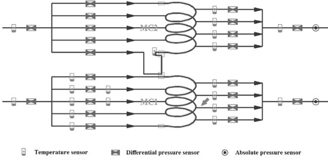
Fig. 2. Calorimetric measurement system arrangement diagram: An arrow points the 112R line, which is used for analysis.
