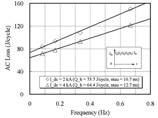
Fig. 5. Frequency spectrum of the total measured AC loss in case of the DC-biased sine wave application:  $I_{ac} = 0.5$  kA.
