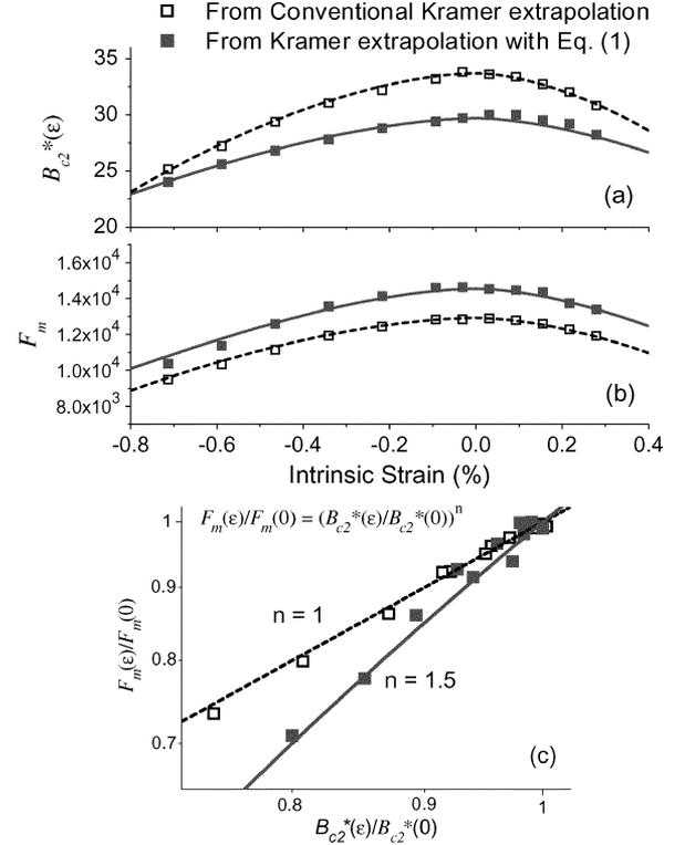
Fig. 6. (a) The extrapolated upper critical field  $B_{c2}^*$  as a function of intrinsic strain. A dotted line is calculated with the scaling law of Ekin and a solid line is calculated with (2). (b)  $F_m$  as a function of intrinsic strain. A dotted line is calculated with the scaling law of Ekin and a solid line is calculated with (3). (c) Log-log plots of the normalized  $F_m$  versus the normalized  $B_{c2}^*$ .
