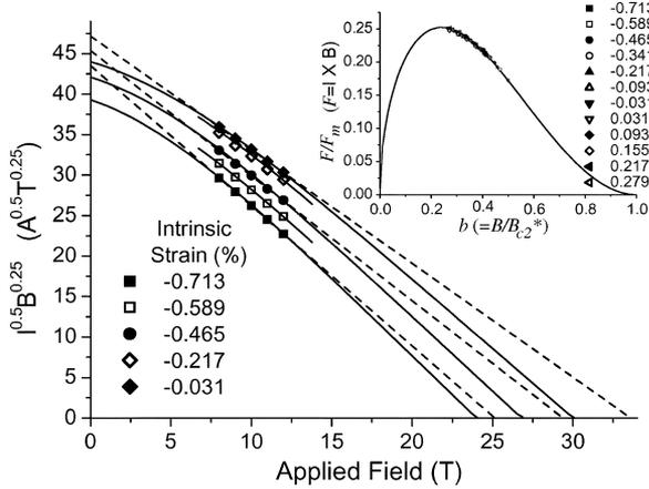
Fig. 5. The Kramer plots for KAT type A. Solid lines are fitting results with (1),  $g = 1.5$ , and dotted lines are the conventional linear extrapolation. Inset: Normalized pinning force versus reduced field.
