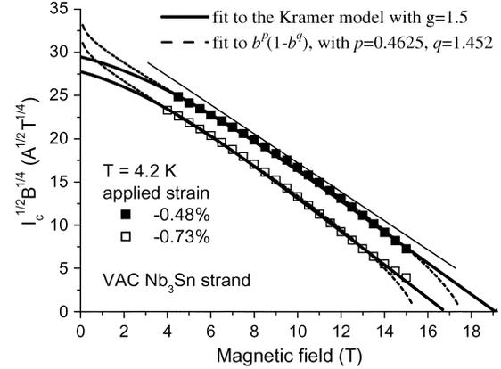
Fig. 3. The Kramer plot of VAC  $\text{Nb}_3\text{Sn}$  strand [8]. Dotted lines are fitting results with a function  $f(b) = b^p(1 - b)^q$  ( $p = 0.4625, q = 1.452$ ). Thick solid lines are obtained from fits to (1), with  $g = 1.5$ .
