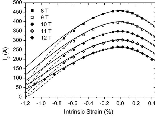
Fig. 4. The critical current as a function of intrinsic strain for KAT Nb<sub>3</sub>Sn strand type A at 4.2 K. Dotted lines are calculated with the strain scaling law of Ekin, and solid lines are calculated with (1), (2) and (3).
