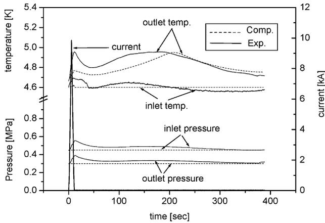
Fig. 7. Comparison of experimental temperature and pressure with those of the computation.
