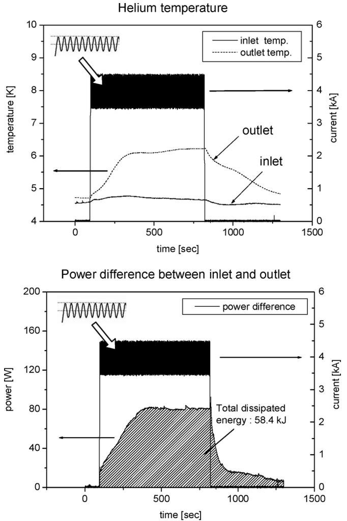
Fig. 3. Helium temperature and power dissipation of AC test.
