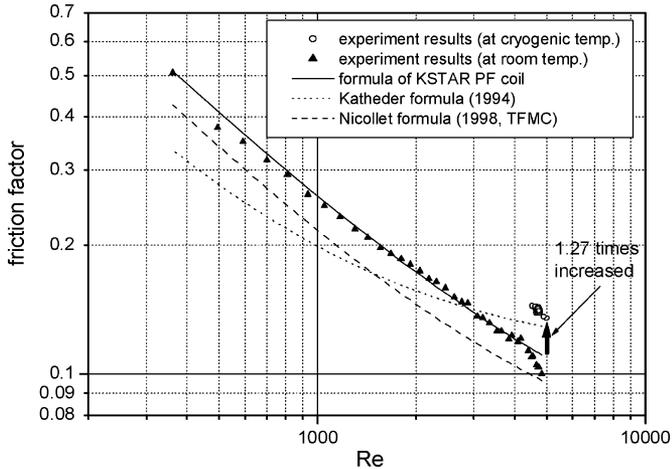
Fig. 5. Comparison of experimental results of CSMC conductor with other experimental results.
