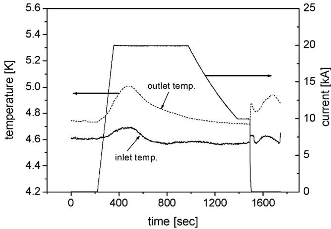
Fig. 2. Helium temperature at inlet and outlet during the DC test.
