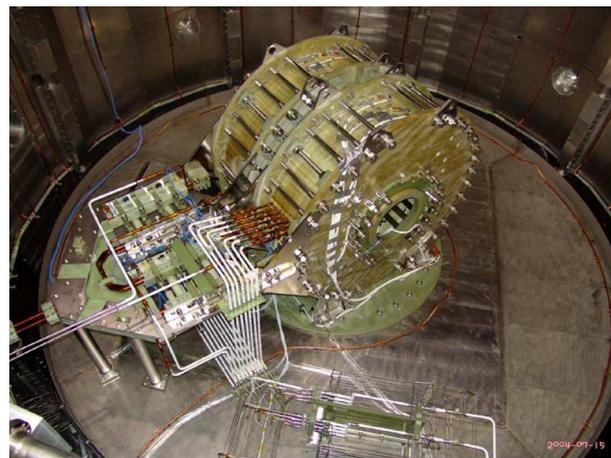
Fig. 1. KSTAR CSMC installed inside the large vacuum cryostat. The coil system consists of two split coils, MC1 and MC2.
