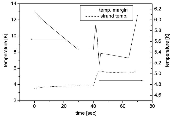
Fig. 9. Temperature margin and strand temperature of KSTAR CS1 coil in a KSTAR reference scenario.
