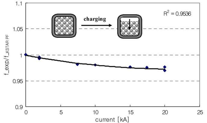
Fig. 6. Variation of friction factor ratio during charging the coil.
