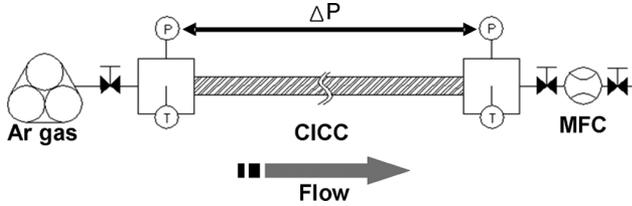
Fig. 4. Friction factor measurement system at room temperature.
