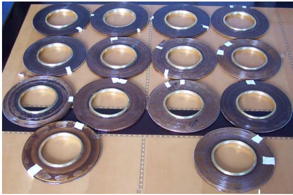
Fig. 1. Coil former and pancake coil.
