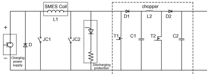
Fig. 5. Topology structure in converter with a two-stage booster.
