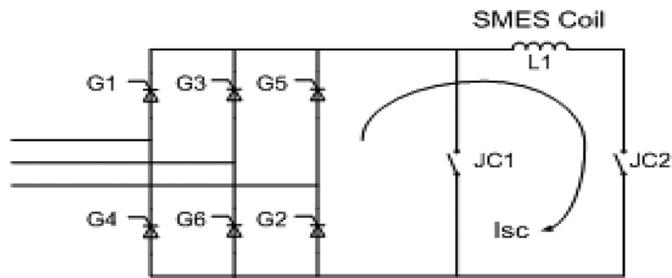
Fig. 6. Charging circuit for superconducting magnetic storage system.
