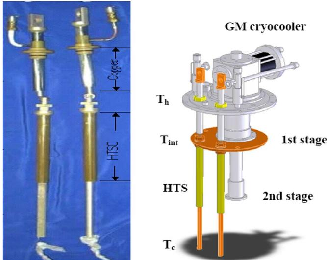
Fig. 4. High temperature current lead for the superconducting magnet.
