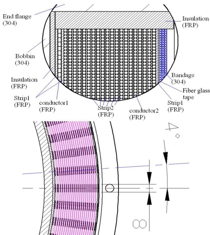
Fig. 1. Configuration of superconducting winding.
