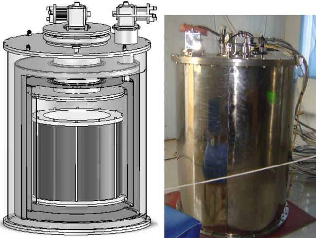
Fig. 3. Overall structure of the cryostat and magnet system.
