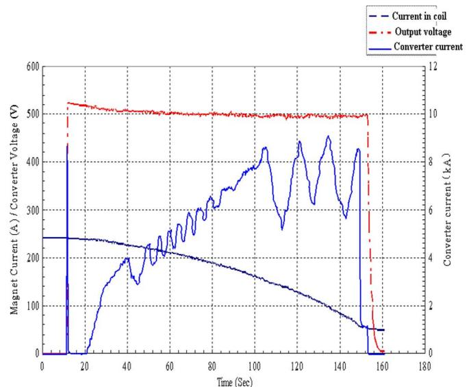
Fig. 9. Profiles of current, output voltage and power in SMES.
