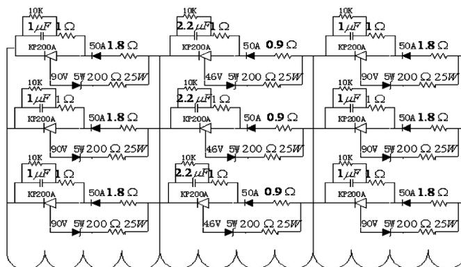
Fig. 2. Protection circuit for superconducting magnet.
