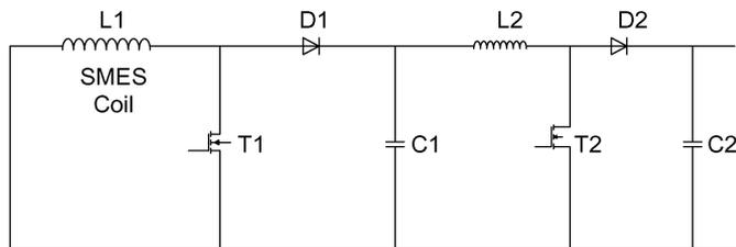
Fig. 7. Topology configuration of a chopper.
