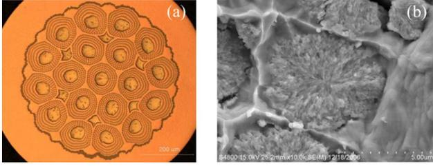
Fig. 3. Optical microscope and FE-SEM images before and after heat treatment for a KAT internal-tin processed Nb<sub>3</sub>Sn strand.
