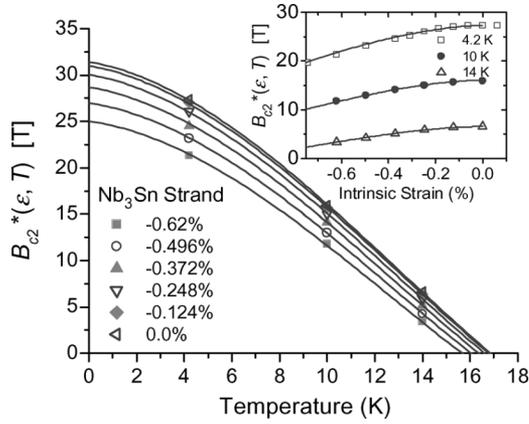
Fig. 6. The extrapolated upper critical field as a function of temperature and strain for the KAT internal-tin processed Nb<sub>3</sub>Sn strand.
