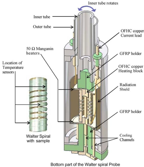
Fig. 1. A schematic cross-sectional view for the bottom part of the variable temperature Walters spiral probe. Inset: A photograph of the Walters spiral with a sample soldered around it.
