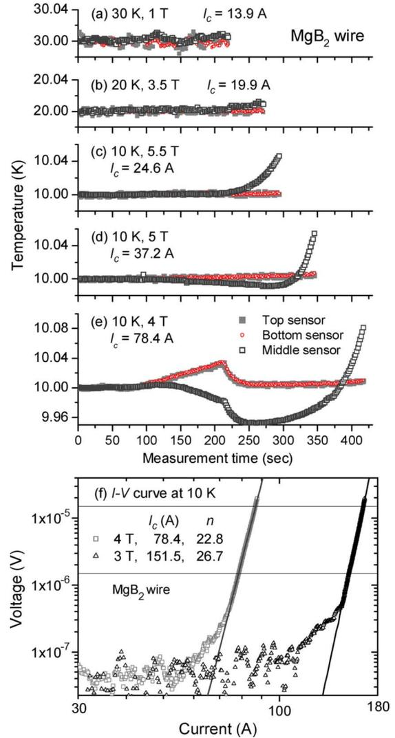
Fig. 2. Temperature fluctuation during the critical current measurement. (f): measured  $I - V$  characteristics for the Hyper Tech  $\text{MgB}_2$  wire.
