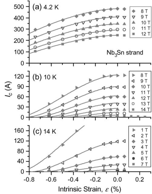
Fig. 4. The field, temperature and strain dependence of the critical current for the KAT internal-tin processed Nb<sub>3</sub>Sn strand.
