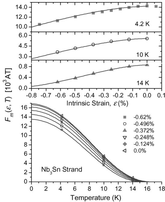
Fig. 7. The pinning force maximum as a function of temperature and strain for the KAT internal-tin processed Nb<sub>3</sub>Sn strand.
