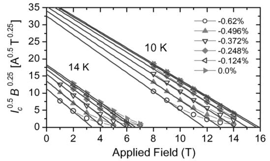
Fig. 5. Kramer plots for the KAT internal-tin Nb<sub>3</sub>Sn strand at 10 and 14 K.
