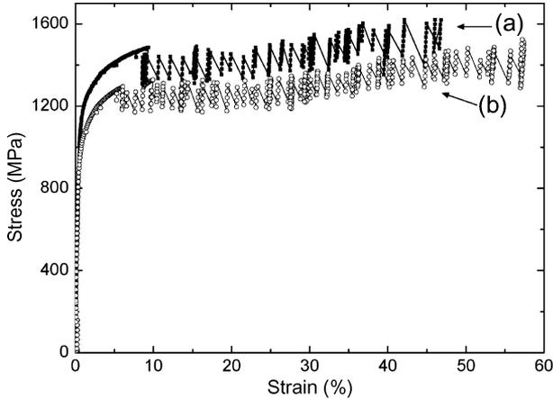
Fig. 2. Tensile test result of KOTF conduit specimens measured at 4.2 K. From top to bottom, (a) compacted and heat treated, 1.9 mm thickness, (b) uncompact and heat treated, 1.6 mm thickness.
