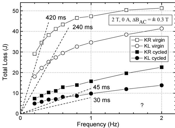
Fig. 5. AC loss measurement result of KOTF samples before and after cyclic load. DC background field was 2 T and  $\pm 0.3$  T alternating field was applied for the measurement.
