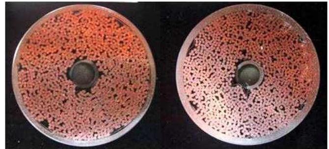
Fig. 1. Cross sectional view of the two KOTF conductors. The estimated void fraction and the conduit tube thickness of the left leg are 33%, 1.6 mm and those of the right leg are 31%, 1.9 mm.
