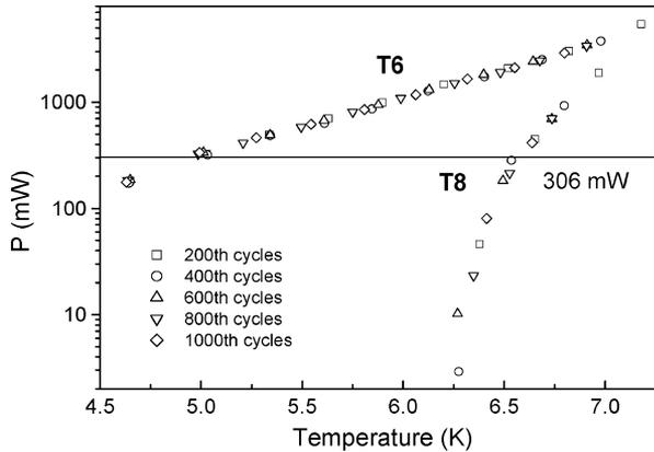
Fig. 4. The steady state He flow calorimetric measurement result of KOTF\_R under cyclic loading. The horizontal line is for power dissipation equivalent to  $10 \mu\text{V/m}$  current sharing electric field.
