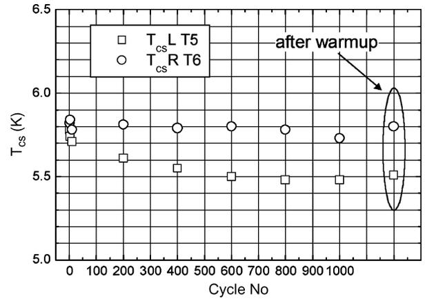
Fig. 3.  $T_{cs}$  evaluation results at several stages between cyclic loads. The left leg (TcsLT5) is 33% void fraction sample and right leg (TcsRT6) is 31% void fraction sample.
