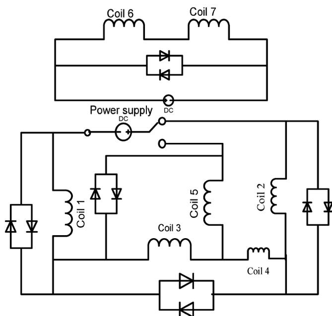
Fig. 4. Quench protection circuit of the superconducting magnet.
