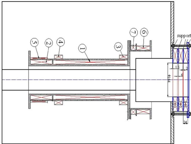
Fig. 1. 10 coils in the magnet have the same axis, the coils are installed in the cryostat, the conventional copper coils are located outside of cryostat and fixed on the flange of the cryostat, they are cooled by air convection. The superconducting coils are cooled by GM cryocooler.
