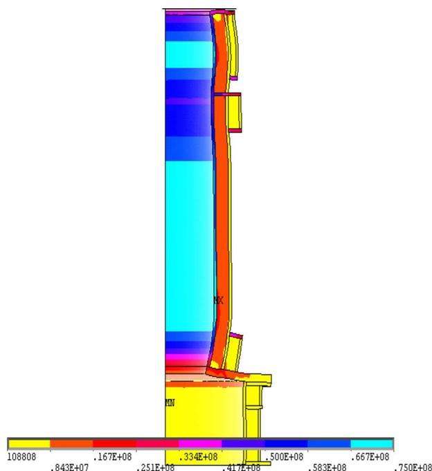
Fig. 3. Stress for superconducting magnet operated at 4 T (Unit:Pa).
