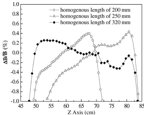
Fig. 6. Measuring results for the magnetic field along  $z$  axis.
