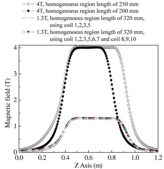
Fig. 2. Magnetic field distribution for various homogeneous region lengths.
