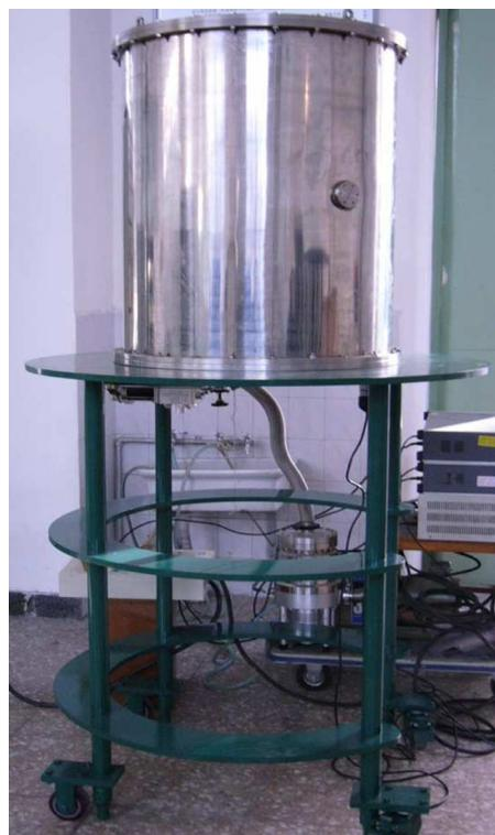
Fig. 5. Configuration for cryostat for the superconducting magnet.
