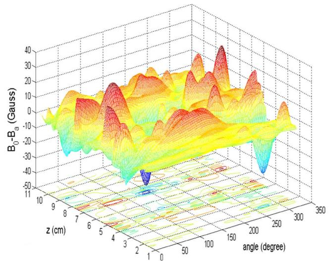
Fig. 7. Measurement results for the magnetic field error along in azimuth direction and  $z$  axis.
