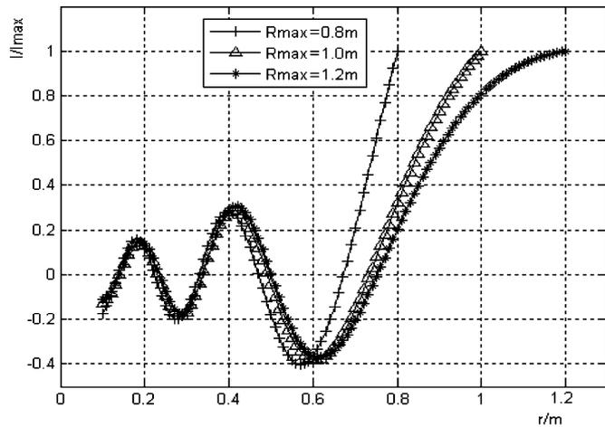
Fig. 3. Normal current distribution for various  $R_{max}$ .
