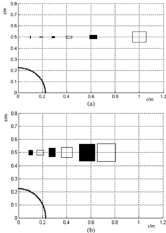
Fig. 4. Configuration of fully open MRI superconducting coils with  $R_{amax} = 1.2$  m (a) and  $R_{max} = 0.8$  m (b).
