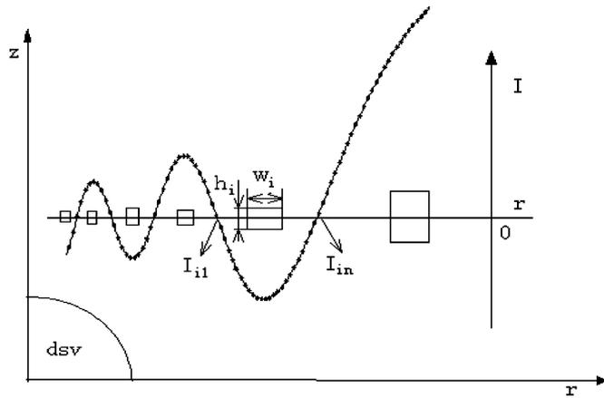
Fig. 1. Schematic of initial dimensions of the coils bulks.
