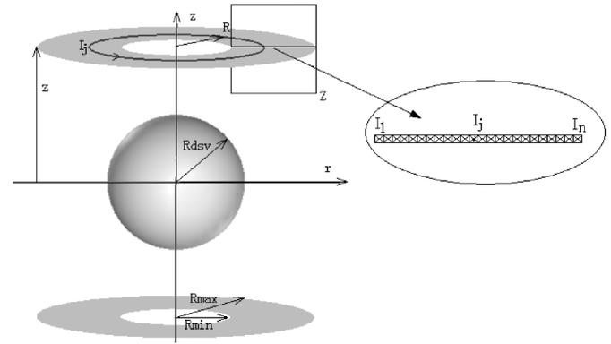
Fig. 2. Discretizing the opened superconducting coils as current loops.
