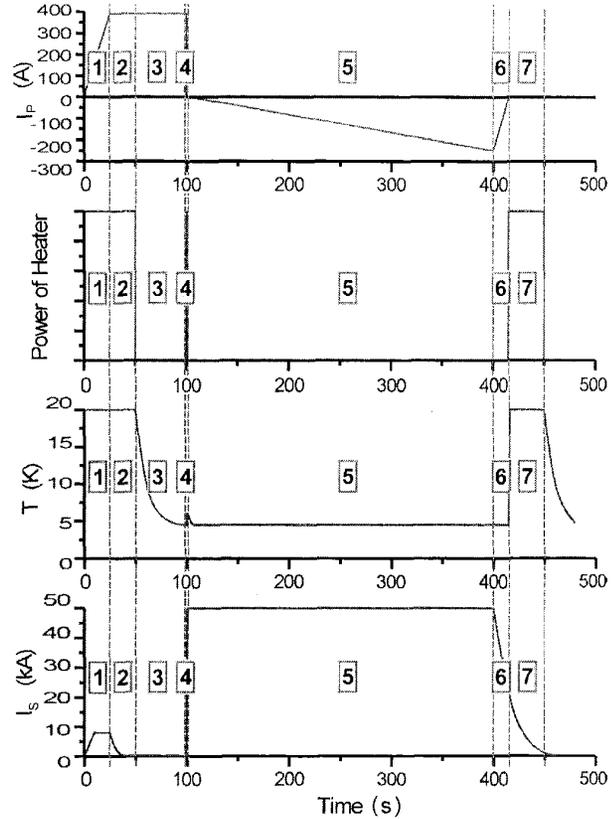
Fig. 2. Typical superconducting transformer duty cycle. Numbers in rectangle denote the operation stages.
