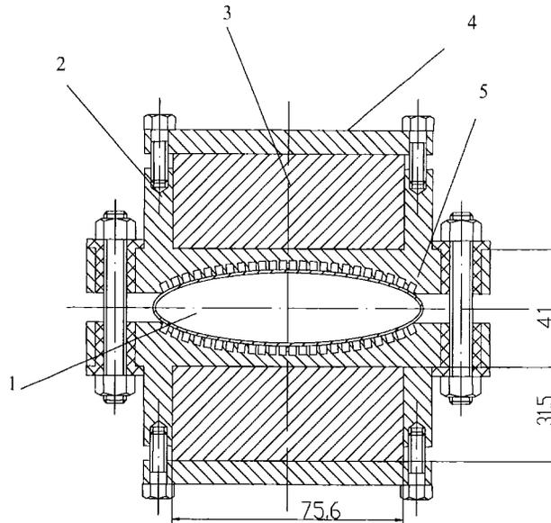
Fig. 5. Design of the joints between the SW-SS ends: 1 – cold finger of the LHe container, 2 – copper mandrel, 3 – copper SS termination, 4 – strengthening plate, 5 – subcable (6 strands) of SW conductor.
