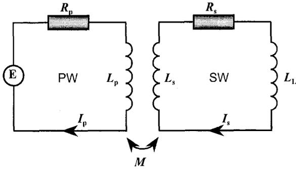
Fig. 1. Schematic circuit of superconducting transformer.
