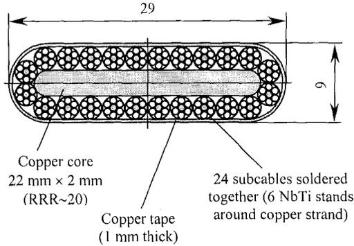
Fig. 3. The secondary winding conductor cross-section (unit: mm).
