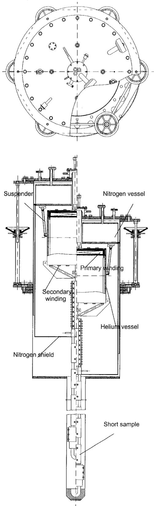
Fig. 4. Superconducting Transformer design; top view and side view. Note that left half drawing shows the upper boundary state of superconducting transformer.
