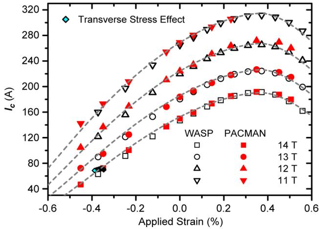
Fig. 4. The strain dependence of the critical current for the internal tin sample. Dotted lines are fitting results using strain scaling law. Solid diamond symbols are converted data from transverse stress measurements.
