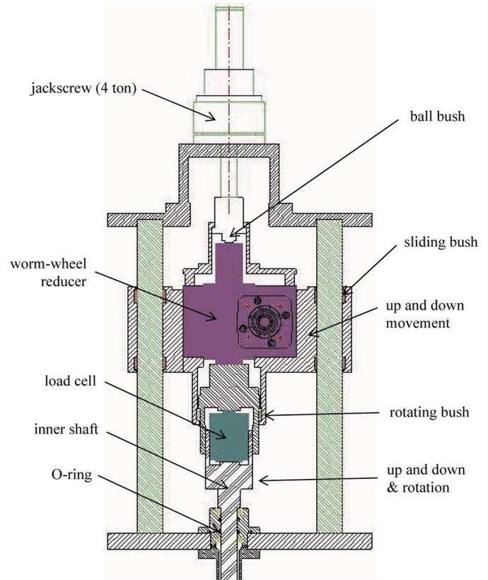
Fig. 2. A schematic diagram for the upper part of the developed apparatus. The inner shaft is attached to the worm-wheel reduce and the worm-wheel reducer is connected with the jackscrew. Both rotational and translational movement is possible.
