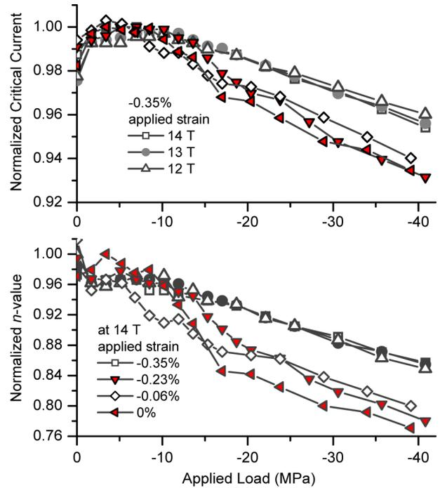
Fig. 5. Normalized critical current and  $n$ -value as a function of applied load at different axial compressive strain and applied field.
