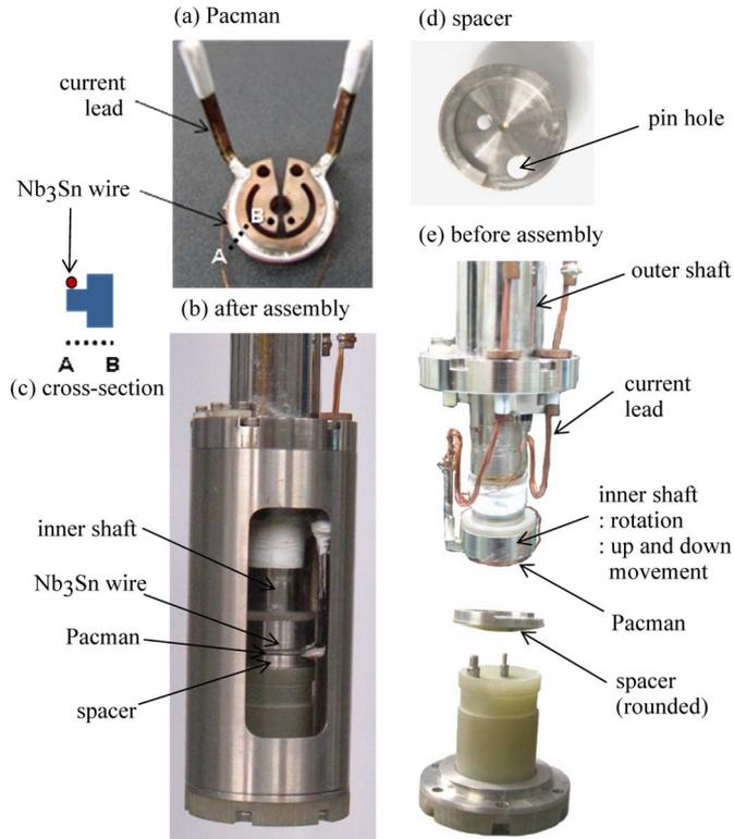
Fig. 1. The bottom part of the developed apparatus. (a) sample soldered on a Pacman, (b) a photograph after assembly, (c) a schematic cross-sectional view, (d) a spacer used for sample adjustment, and (e) a photograph before assembly. GFRP was used for electrical insulation.
