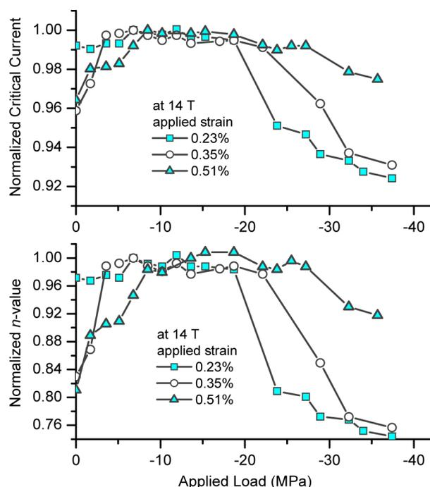
Fig. 6. Normalized critical current and  $n$ -value as a function of applied load at different axial tensile strain.
