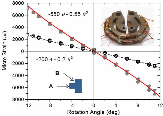
Fig. 3. Angular dependence of strain measured from the attached strain gages. (inset) A photograph after strain gage attachment.
