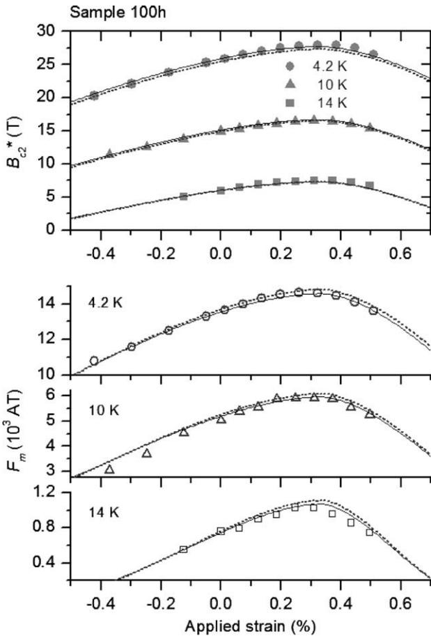
Fig. 5. The pinning force maximum as a function of temperature and strain for the sample 100 h.
