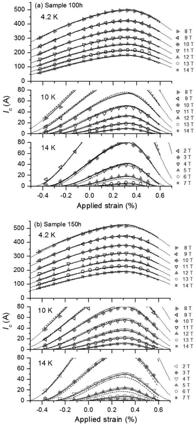
**Fig. 2.** The field, temperature and strain dependence of the critical current for the KAT internal-tin processed Nb<sub>3</sub>Sn strand with different heat treatment scenarios. Solid lines were calculated with Eq. (2), the scaling law based on strong-coupling theory and dotted lines were calculated with Eq. (3), the modified deviatoric scaling law.
