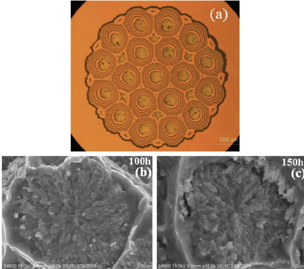
Fig. 1. Optical microscope and FE-SEM images before and after heat treatment for a KAT internal-tin processed Nb<sub>3</sub>Sn strand.
