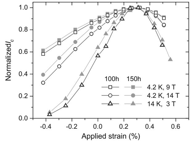
**Fig. 3.** Normalized  $I_c$  as a function of applied strain for the samples 100 h and 150 h at various fields and temperatures.
