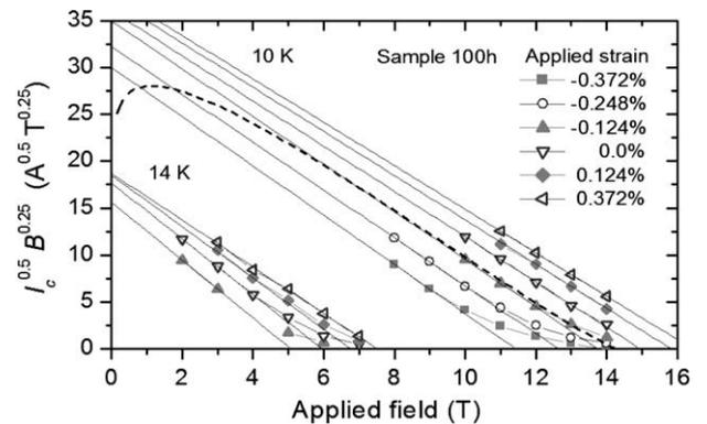
**Fig. 4.** Kramer plots for the sample 100 h at 10 and 14 K. Solid lines are the Kramer extrapolations and the dotted line corresponds to  $b^{0.697}(1-b)^{2.266}$ .
