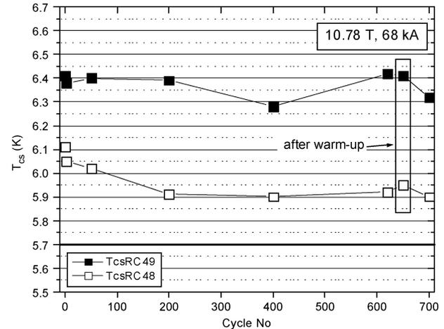
Fig. 3.  $T_{cs}$  versus number of cyclic loads for RC48 and RC49 sample, the horizontal line at 5.7 K is the acceptance criterion.
