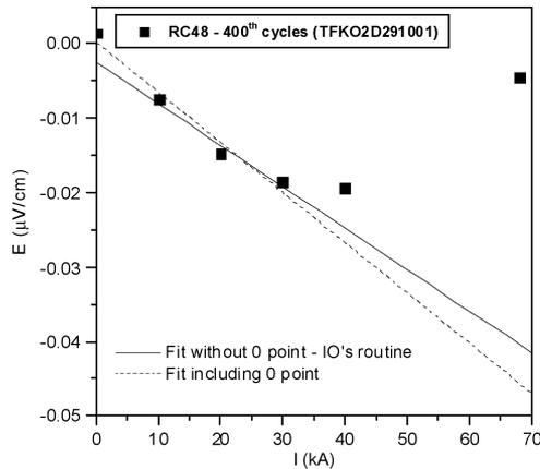
Fig. 2. Here is an illustration of the IO's standard method for linear extrapolation to compensate early voltage. The solid line is the same way in IO's routine comparing with the deviation from another linear fitting of dashed line including the zero point.
