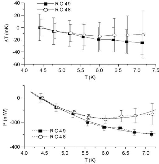
Fig. 4. The thermal background of calorimetric measurement is given in this figure. The temperature differences without current will be interpreted as a background heat power which had to be subtracted from the data, temperature vs. power. The standard deviation of 4 sensors was regarded as the statistical error which can be employed to estimate the error of power with the error propagation formula of  $\sigma_p^2 = (C_{p2}^2 \sigma_{T2}^2 - C_{p1}^2 \sigma_{T1}^2)(dm/dt)^2$ .
