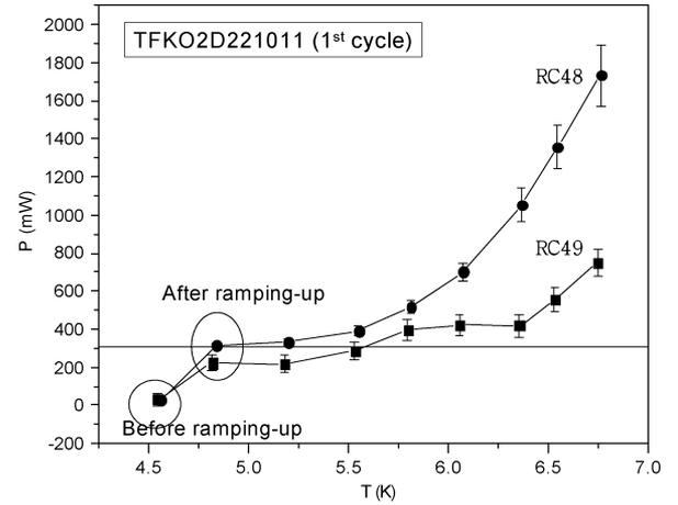
Fig. 5. Temperature versus Joule heat power without any correction of initial offset after the compensation of thermal background (1st cycle).
