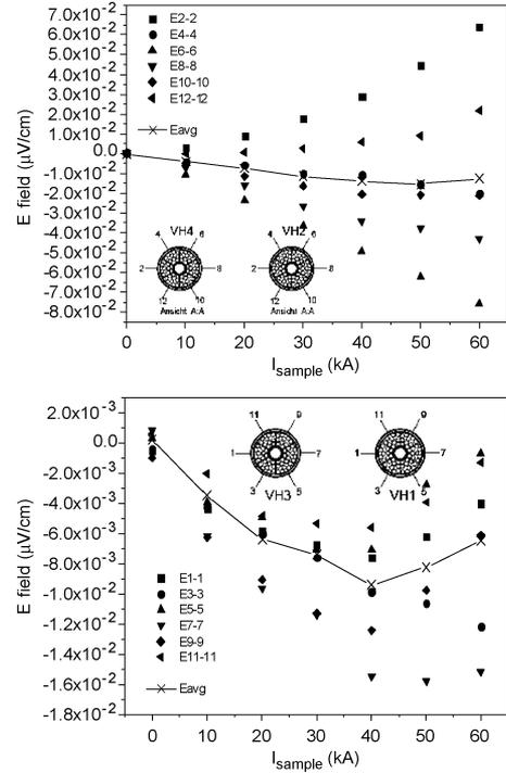
Fig. 1. The maximum level of early voltage (for averaged signal) is about 10% ~ 20% of the voltage criterion for  $T_{cs}$  assessment. The early voltages from the individual V-tap pairs are presented for RC48 right leg (upper) and RC49 left leg (lower).
