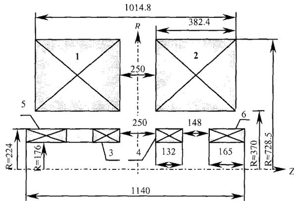
Fig. 3. Geometry of MC+BCC: 1,2 - main coils, 3,4 - blip coils, 5,6 - cancellation coils (unit: mm).
