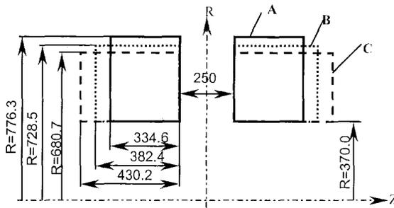
Fig. 1. The comparison of geometry of MC for optimization (unit: mm).
