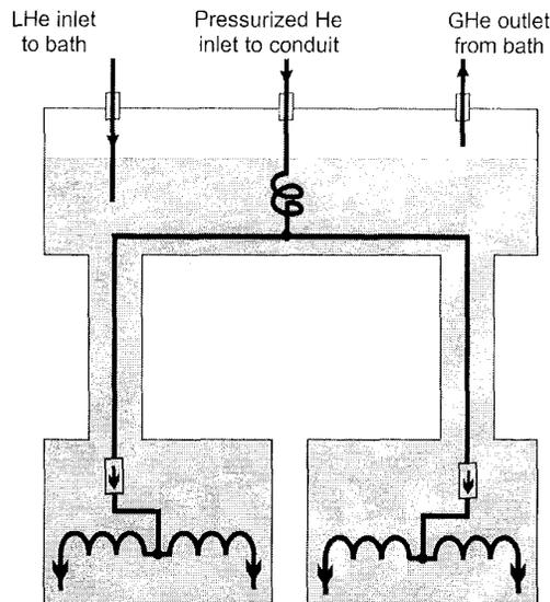
Fig. 5. Hydraulic layout of BCC.
