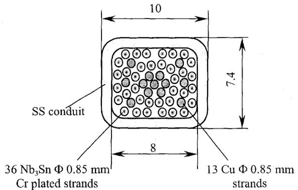
Fig. 4. BCC conductor cross-section (unit: mm).
