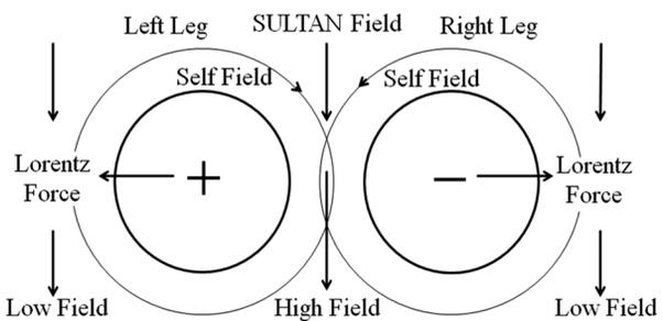
Fig. 4. Top view of the magnetic field configuration. A combination of the background field and the self field produces the field gradients.
