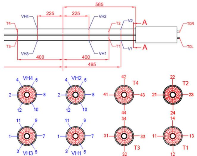
Fig. 1. Instrumentation of the TFKO3 sample. Lower conductor is the *left leg*, and the upper conductor is the *right leg*. The distance between voltage taps is 0.45 m. The lower diagram illustrates the location of voltage taps and temperature sensors as viewed from the top of the samples in SULTAN.
