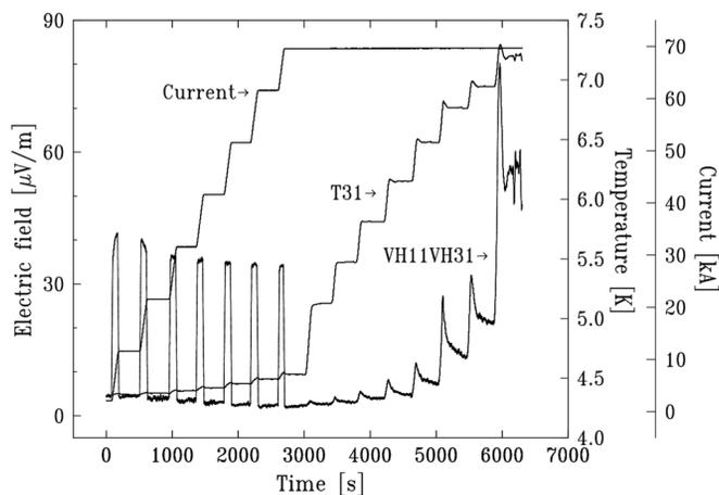
Fig. 2. Voltage (VH11VH31), temperature (T31), and current during a  $T_{cs}$  run at the first cycle ( $N = 1$ ). Electric field is obtained from the voltage divide by the distance between voltage taps, 0.45 m. All the signals were centered averaged for 501 data points.
