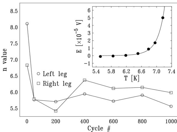
Fig. 6. Evolution of the  $n$  value of the left and right legs. Connecting lines are for guidance only. The inset shows the electric field of the left leg versus temperature at  $N = 1$ . The curve in the inset is the fitted result of the electric field to (1).
