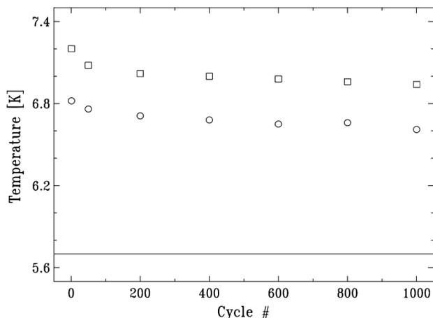
Fig. 3. Evolution of  $T_{cs}$  up to the cycle 1000. Circles and squares represent the  $T_{cs}$  of the left and right legs respectively. The acceptance criteria, which is 5.7 K is shown with a solid line.
