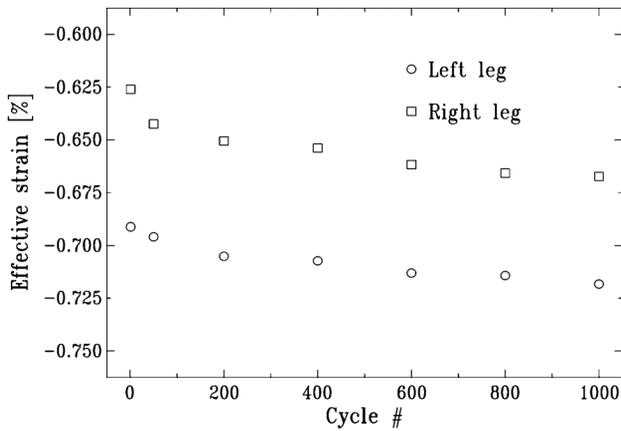
Fig. 5. Evolution of the effective strain of the left and right legs.
