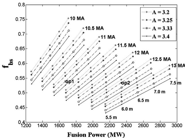
Fig. 1. The bootstrap current fraction and the fusion power for conventional magnetic shear case, with various aspect ratios of 3.2–3.4 and plasma currents in the range of 10–13 MA.
