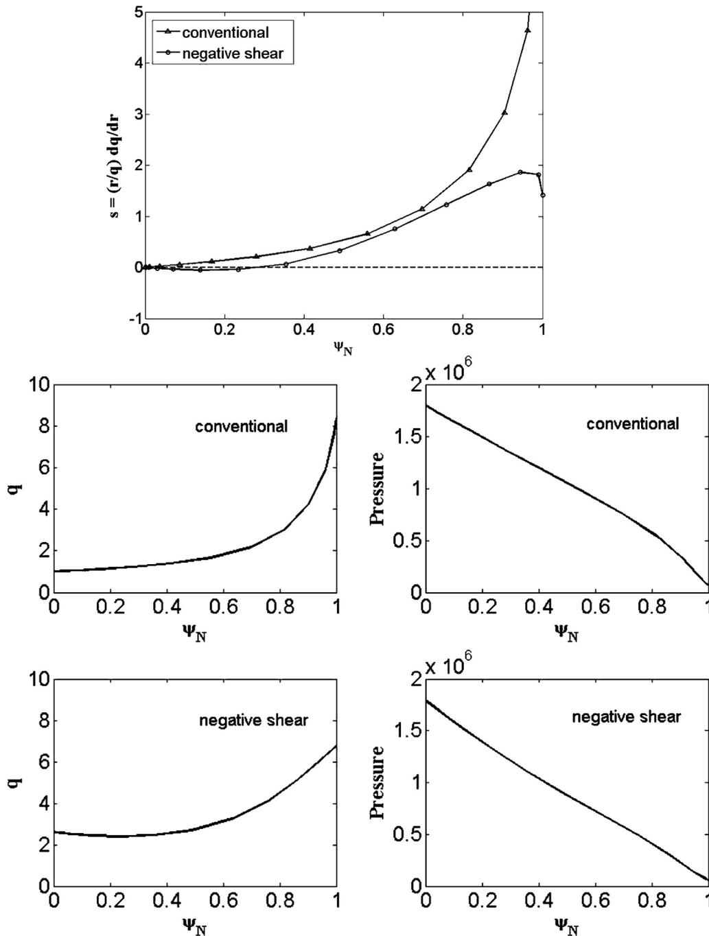
Fig. 3. The safety factor, pressure, and magnetic shear  $s = (r/q) dq/dr$  profiles for the conventional magnetic shear (triangles) and negative shear cases (circles).
